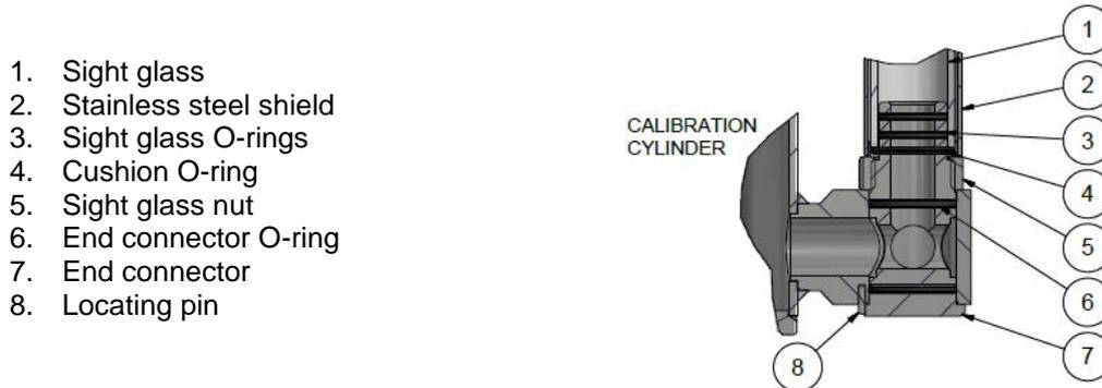
Cleaning the inside of the sight glass contained within the Stainless steel shield is as follows:
