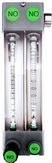
Series 1241S Dual Tube Cascade Flowmeter Where a wide turndown ratio is required, this instrument can cascade two flow tubes to give accurate readings with a 100:1 turndown.
