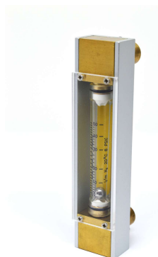
Series 1241S Dual Tube Cascade Flowmeter Where a wide turndown ratio is required, this instrument can cascade two flow tubes to give accurate readings with a 100:1 turndown.
