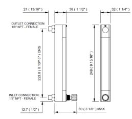
**STANDARD OXYGEN FLOW RATES:** 0.1-4 L/min 02 @ 1013 mbar abs 20°C, 0.1-8 L/min 02 @ 1013 mbar abs 20°C , 0.1-10 L/min 02 @ 1013 mbar abs 20°C
